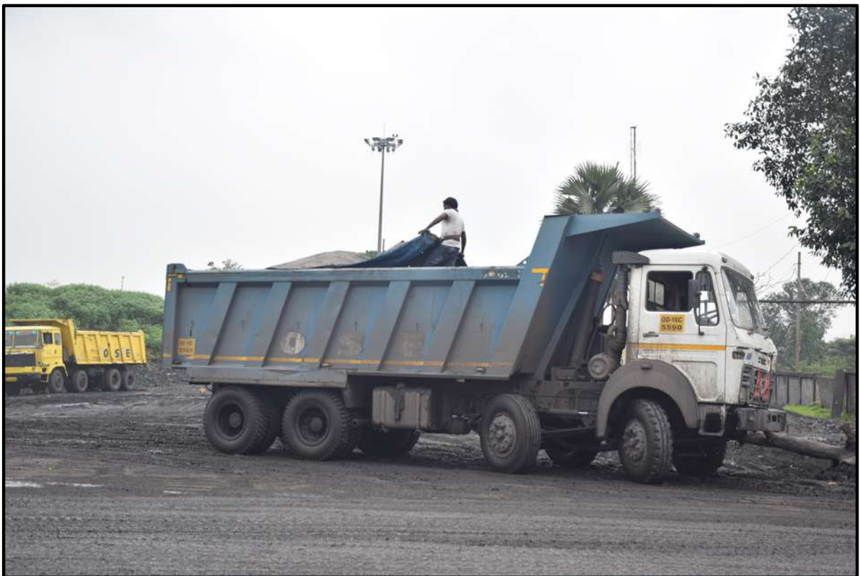
Before transporting coal by road, they are covered by tarpaulin sheets.
